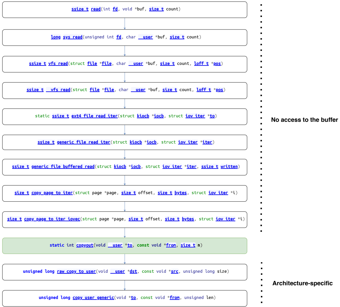
Figure 5.2: A subset of the read path in the Linux kernel. The copyout() function is a viable candidate since it offers access to the kernel buffer containing raw data, and copies it to the user buffer
